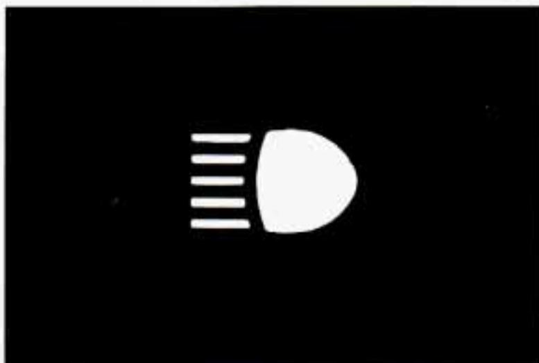
This blue high beam indicator light is above the engine oil temperature gage on the instrument cluster and is on whenever you use your high beam headlamps. See “Headlamp High–Low Beam Changer” in this section.
